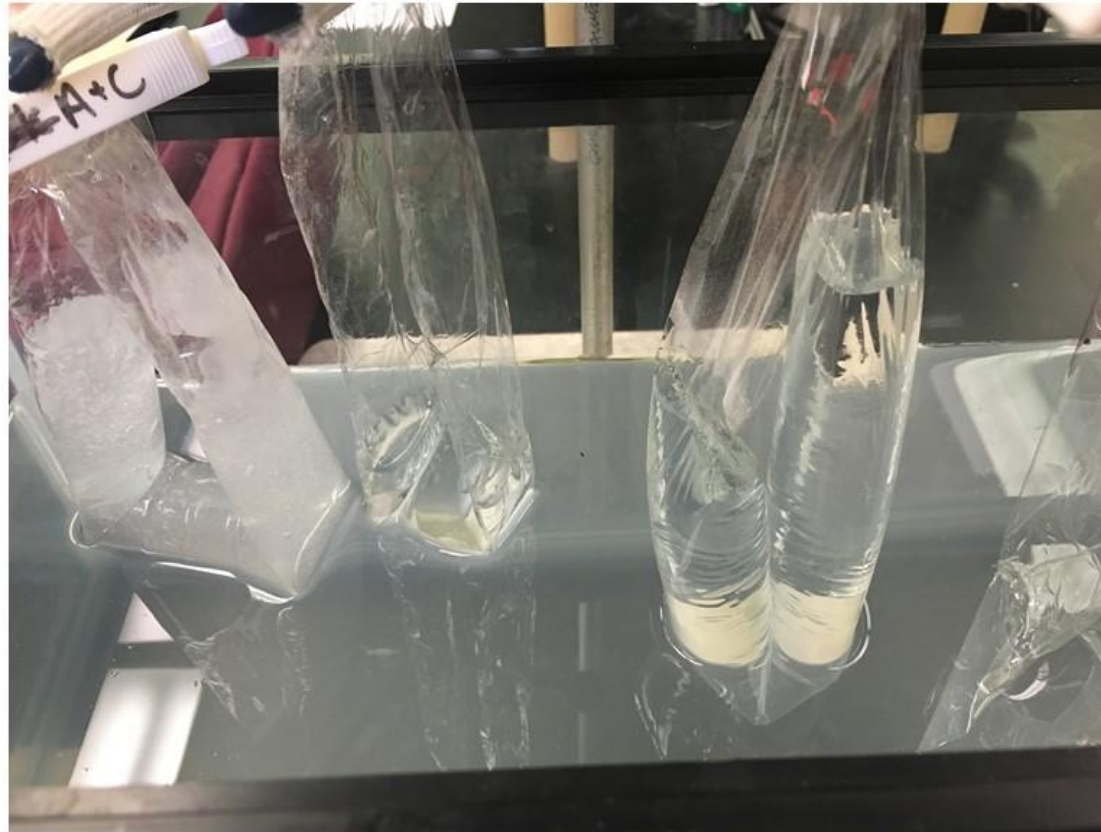
Figure 2: The osmotic pressure experiment described in figure 1. The photograph was taken 48 hours after initially dangling the dialysis tubes into the water. From left to right the dialysis tubes contained 1 gram each of Sodium Acrylates Crosspolymer, Hydroxyethylcellulose, Sodium Carboxymethylcellulose, and common salt. The membrane with common salt collapsed as the salt diffused into the reservoir.
